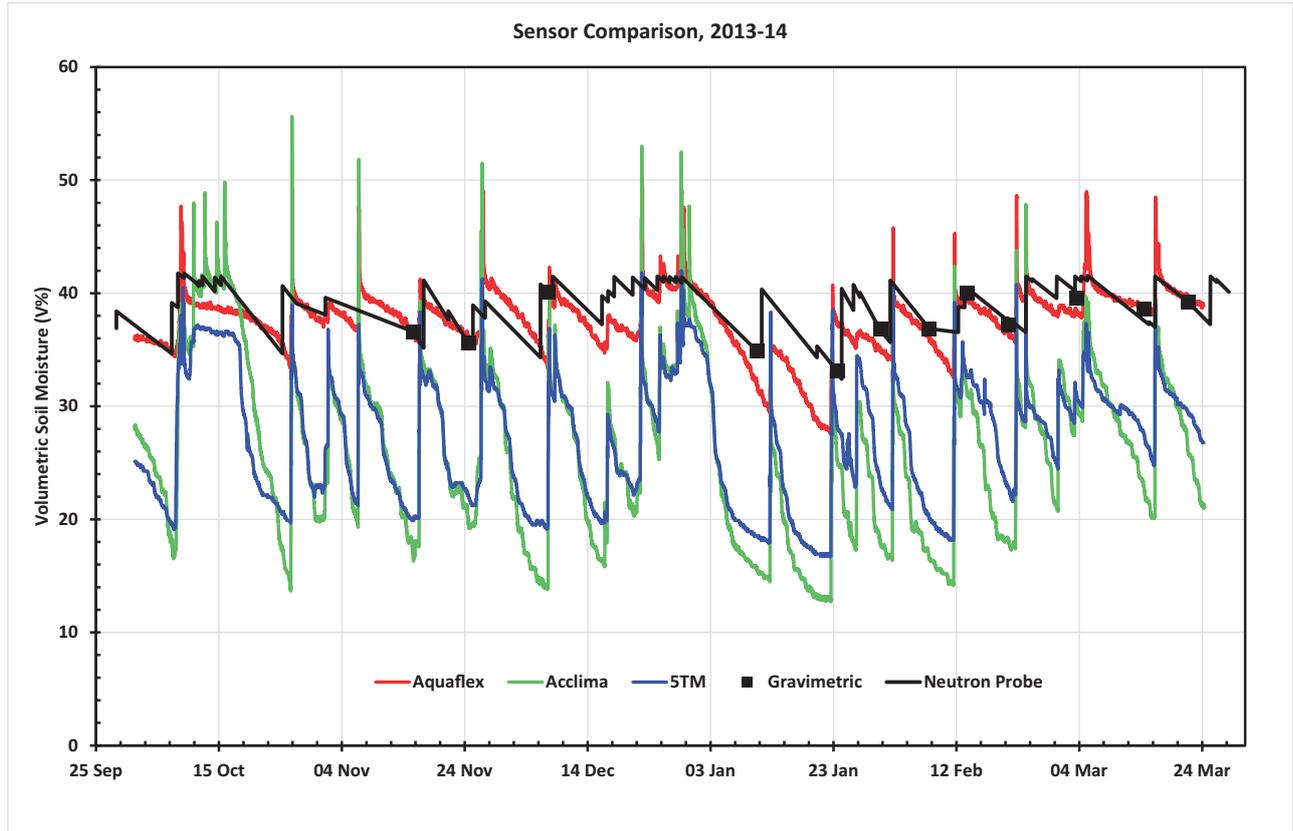
*Comparison of soil moisture sensors in a silt loam soil, Canterbury, New Zealand*
